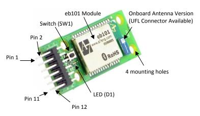
The eb301 features a pin out that provides access to the primary features of the eb101 module.
